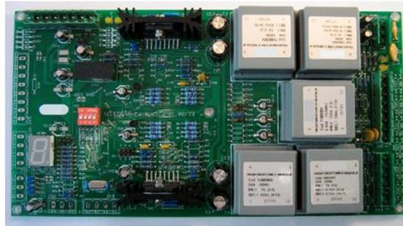
NSI12-02 NMEA - SYNCHRO Interface board is a conversion unit from digital data on serial line to 2 analog signals in synchro format on independent or correlated channels. Multiple operative modes: by means of dip-switches different NMEA sentences and Synchro gear ratio can be selected.
