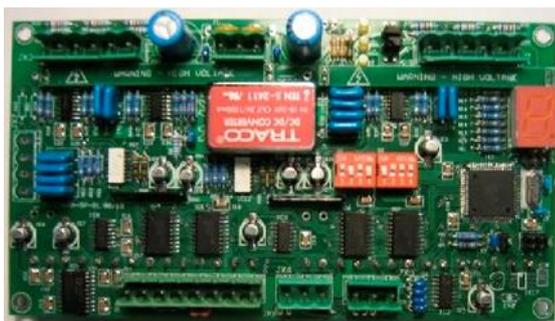
The SNI - API electronic card is a Synchro signals acquisition unit, data processing and transmission on serial line. The primary application is in marine environment (on board installation) in interfacing devices and sensors with output in synchro signals, single and dual-speed (1x/2x + 36x), data conversion and digital distribution with transmission protocol MNEA 0183 (IEC 61162-1), electrical format opto-isolated RS422 or RS232.
